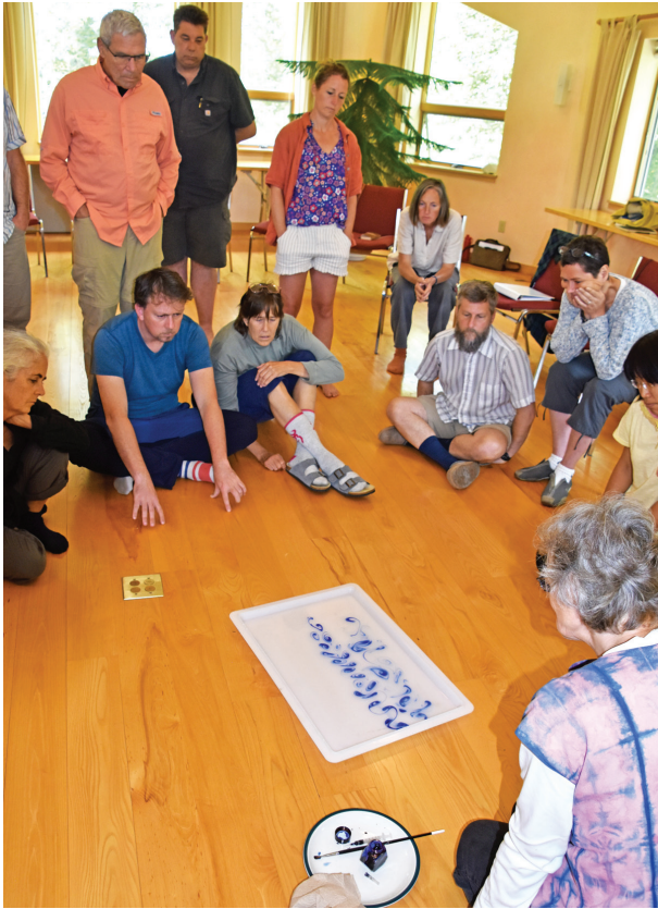
Creating vortex trains in a shallow container by moving a stick straight through drops of ink in sugar water.
