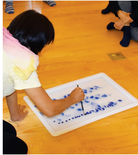
Creating vortex trains in a shallow container by moving a stick straight through drops of ink in sugar water.
