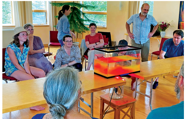
Cold colored water billows upward as it is warmed from below with a heat lamp.
